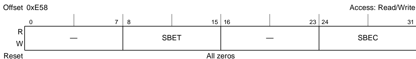
Figure 9-30. Single-Bit ECC Memory Error Management Register (ERR_SBE)
