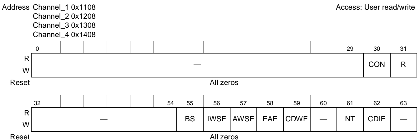
Figure 14-60. Crypto-Channel Configuration Register (CCCR)
