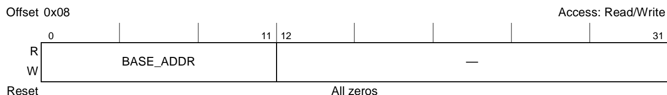
Figure 5-3. Alternate Configuration Base Address Register (ALTCBAR)
