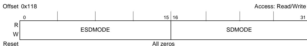
Figure 9-10. DDR SDRAM Mode Configuration Register (DDR_SDRAM_MODE)
