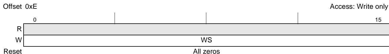
Figure 5-30. System Watchdog Service Register (SWSRR)
