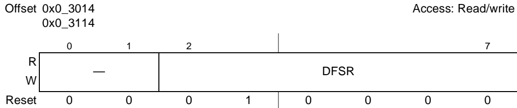
Figure 15-7. I 2 Cn Digital Filter Sampling Rate Register (I2CnDFSRR)
