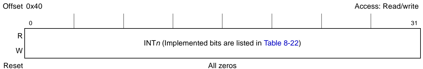
Figure 8-16. System Error Status Register (SERSR)
