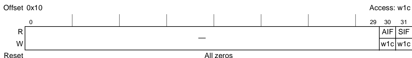
Figure 5-38. Real Time Counter Event Register (RTEVR)
