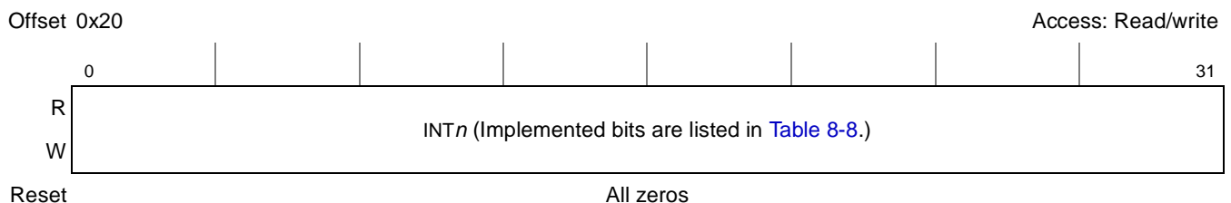
Figure 8-8. System Internal Interrupt Mask Register (SIMSR_H)
