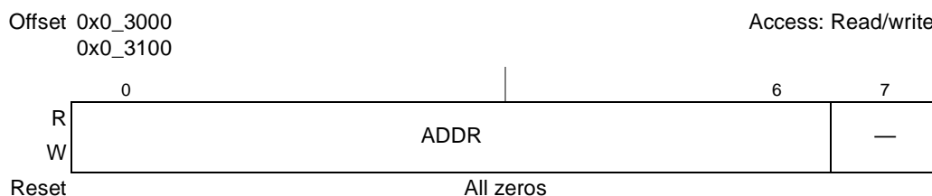
Figure 15-2. I 2 C n Address Register (I2CnADR)
