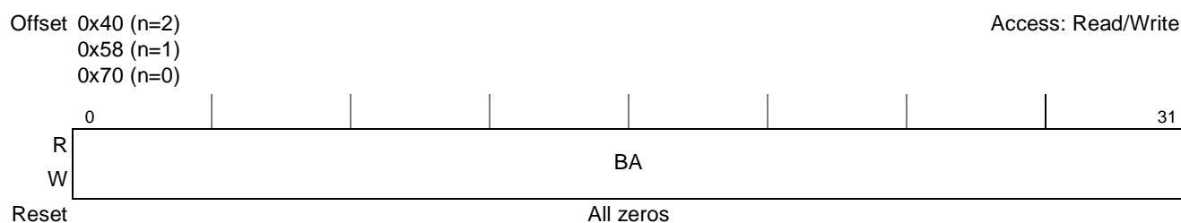
Figure 13-16. PCI Inbound Base Address Registers (PIBAR n )
