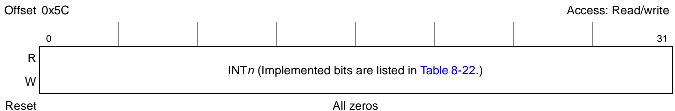
Figure 8-22. System Error Status Register (SERFR)
