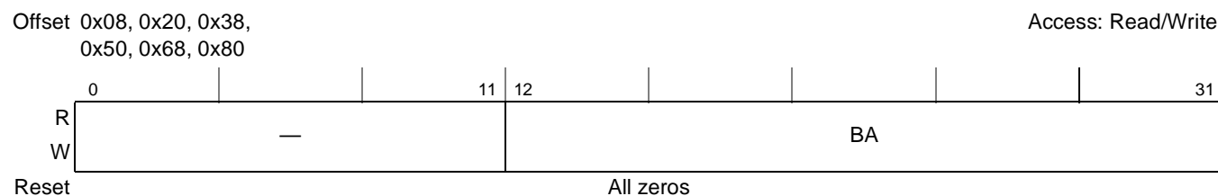
Figure 11-3. PCI Outbound Base Address Registers (POBAR n )
