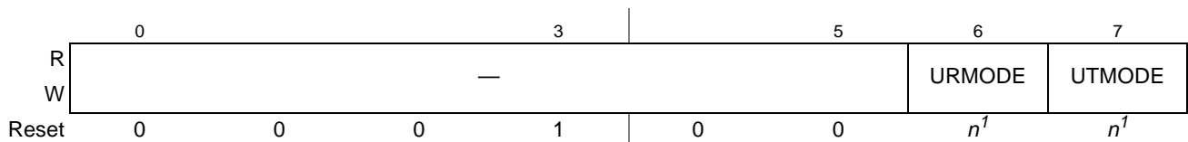
Figure 23-2. General UCC Extended Mode Register
