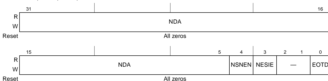
Figure 12-16. DMA Next Descriptor Address Register (DMANDAR n )
