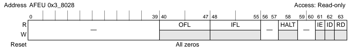
Figure 14-29. AFEU Status Register
