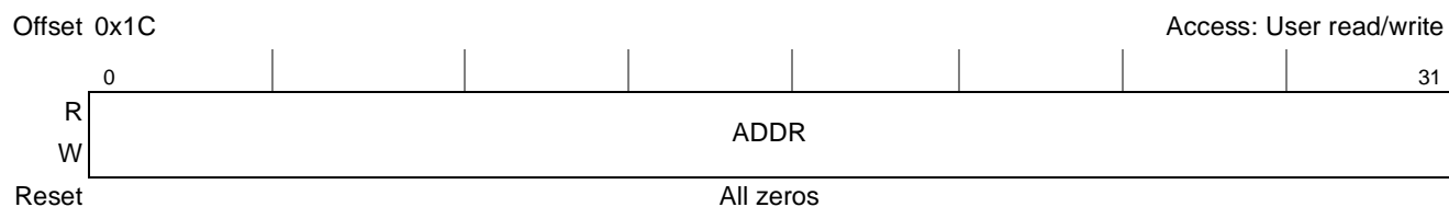
Figure 6-7. Arbiter Event Address Register (AEADR)
