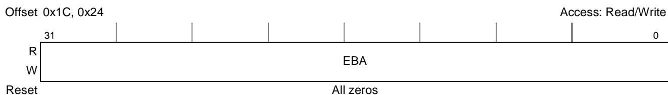
Figure 13-34. GPL Extended Base Address Registers 1–2
