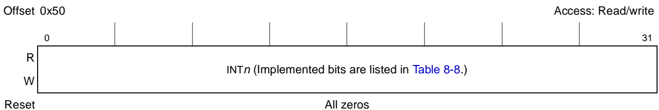
Figure 8-19. System Internal Interrupt Force Register (SIFCR_H)
