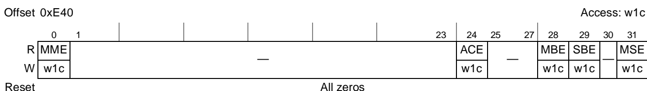
Figure 9-25. Memory Error Detect Register (ERR_DETECT)
