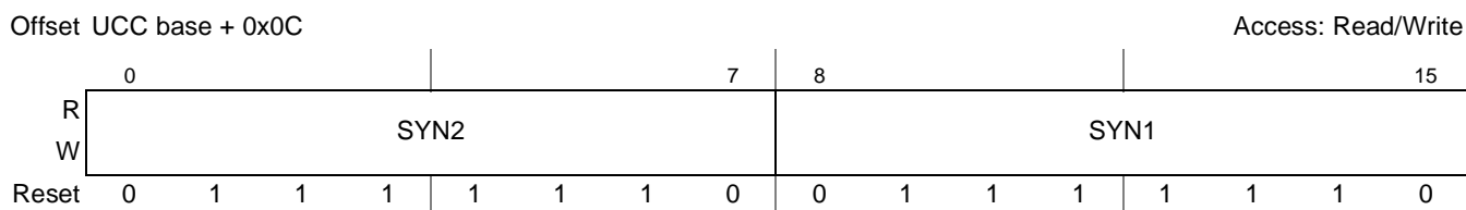
Figure 27-3. UCC Data Synchronization Register (Fast Protocols)
