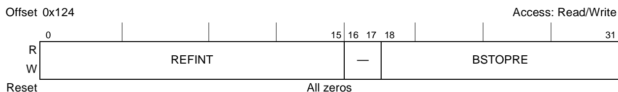
Figure 9-13. DDR SDRAM Interval Configuration Register (DDR_SDRAM_INTERVAL)
