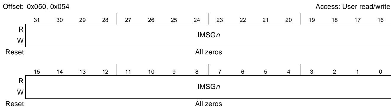
Figure 12-4. Inbound Message Registers (IMR0, IMR1)
