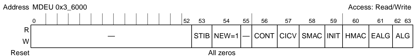
Figure 14-34. MDEU Mode Register (MDEUMR) in ‘New’ Configuration
