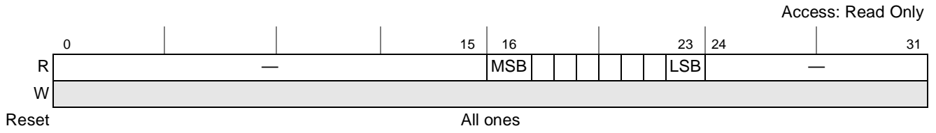
Figure 22-24. SPIRD in REV=0 LEN=0x7
