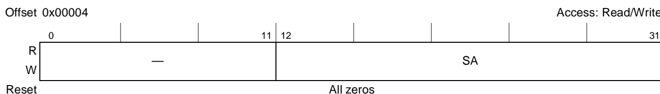
Figure 5-13. Secondary DDR Memory Controller Start Address Register (SDMCSAR)
