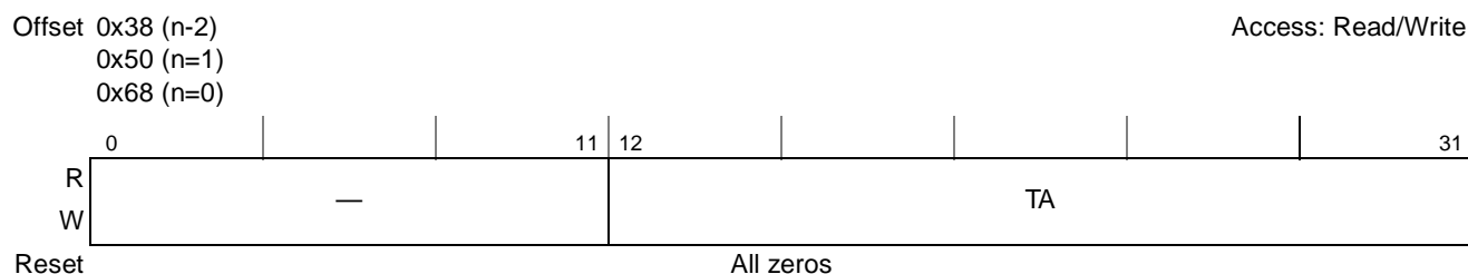
Figure 13-15. PCI Inbound Translation Address Registers (PITAR n )
