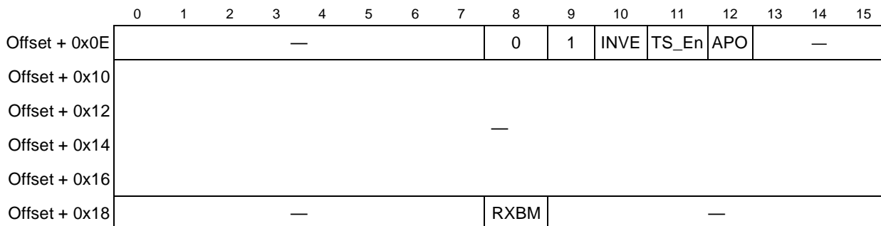
Figure 32-39. AAL0 Protocol-Specific RCT
